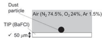
Fig. 2 Geometry of the dust and TIP during TIPT
