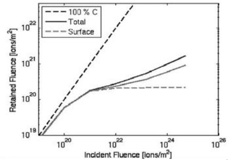
Fig.3 Retained fluence as a function of the incident fluence: the dashed black line corresponds to 100 % retention, the dashed pink curve to a massive sample, the full lines to porous CFC NB31 (the pink curve is the near surface retention; the blue curve is the total retention, including the porous network).
