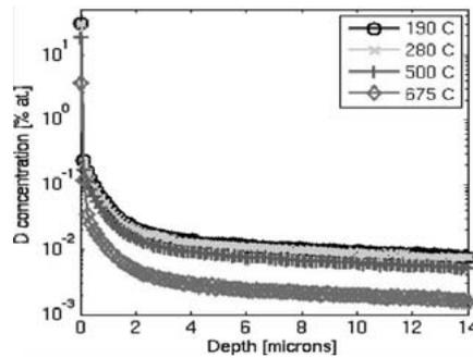
Fig.2 Simulated deuterium concentration profile of CFC NB31 irradiated by 200 eV D<sup>+</sup> ions as a function of sample temperature (middle), for a fluence of  $2 \times 10^{24}$  D/m<sup>2</sup>.
