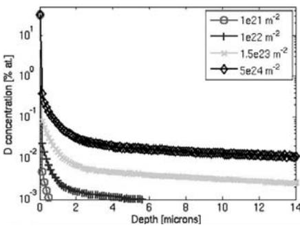
Fig.1 Simulated deuterium concentration profile of CFC NB31 irradiated by 200 eV D<sup>+</sup> ions as a function of incident fluence. Samples are at a temperature of 50 °C.
