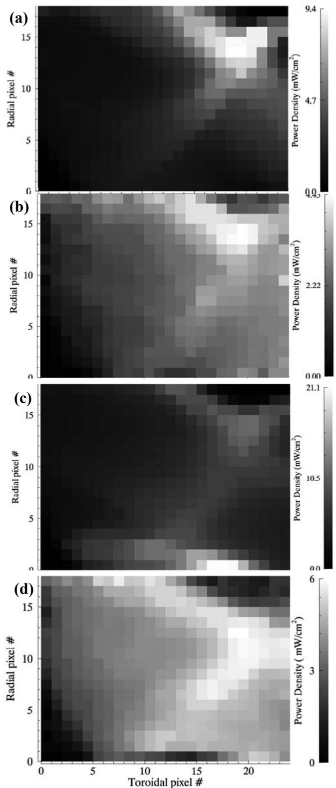
Fig. 1. Synthetic images of radiation from carbon radiation as predicted by EMC3/EIRENE at the upper port IRVB on LHD for densities of  $4.0$  (a),  $6.0$  (c)  $\times 10^{19}/\text{m}^3$  and corresponding experimental IRVB images (18 x 24 channels) of radiated power density from shot #115095 at line averaged densities of  $4.2$  (b) and  $6.0$  (d)  $\times 10^{19}/\text{m}^3$ .
