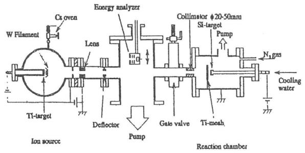
Schematic view of experimental set up
