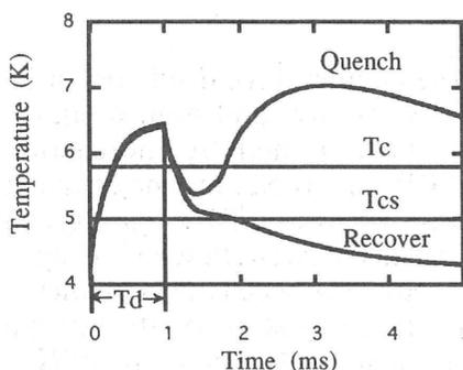
Fig. 2 Time variation of calculated conductor temperature at the center of disturbance
