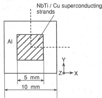
Fig.1 Cross-section of model conductor
