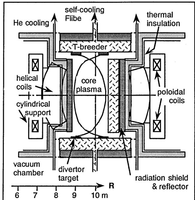
Fig. 1 Schematic illustration of FFHR-2.
