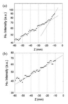
Fig. 2 Ha line intensity as a function of length in Z direction (X=0) from the target. (a) tungsten target and (b) carbon target.
