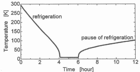
Fig.1 The temperature at the extruding position during the cooling-down and paused phase.
