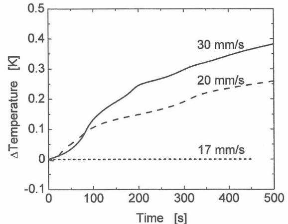
Fig.2 The temperature increase for different extrusion speeds. The base line temperature is 10.5-11 K.
