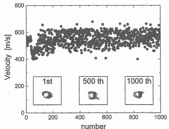
Fig.3 The demonstration of 1000 launches at 10 Hz. The velocity and a typical shadow graph of pellets are shown.
