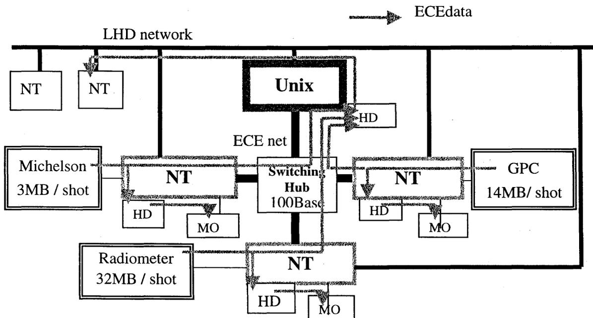
Fig.1 The schematic draw of the ECE data acquisition system .
