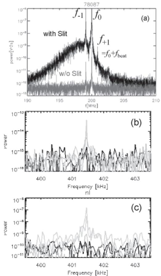
Fig. 2 Power spectrum of the signals from RF pickup coils (a), low frequency pickup coil (b) and microwave interferometer (c). The different colors in Figs. (b), (c) represent difference of the analyzed time window.
