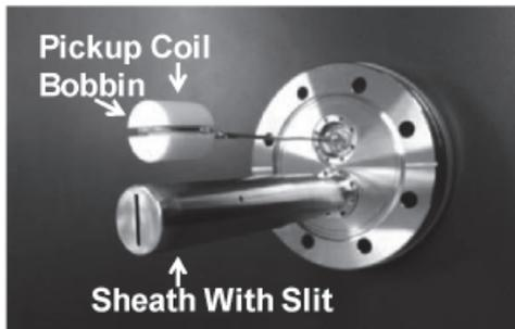
Fig. 1 Photograph of two RF pickup coils, where the stainless sheath of the upper coil was removed to show the inner structure.
