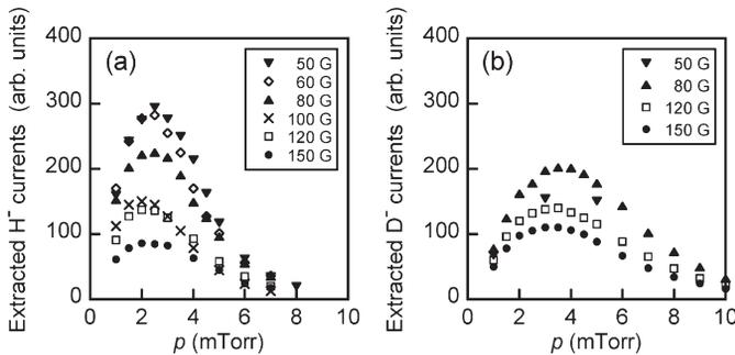
**Fig. 1.** Pressure dependences of extracted (a) H<sup>-</sup> and (b) D<sup>-</sup> currents. Experimental conditions are as follows:  $V_d = 70$  V,  $I_d = 5$  A, and extraction voltage  $V_{ex} = 1.5$  kV. Parameter is the magnetic field intensity of the MF.
