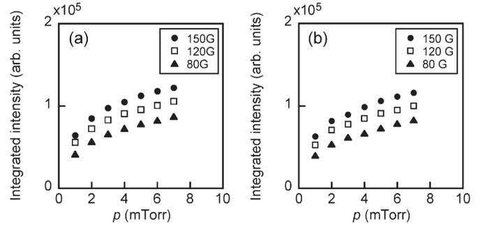
**Fig. 2.** Pressure dependence of integrated intensities of VUV spectra from (a) H<sub>2</sub> and (b) D<sub>2</sub> plasmas, where  $V_d = 70$  V and  $I_d = 5$  A. Parameter is the magnetic field intensity of the MF.
