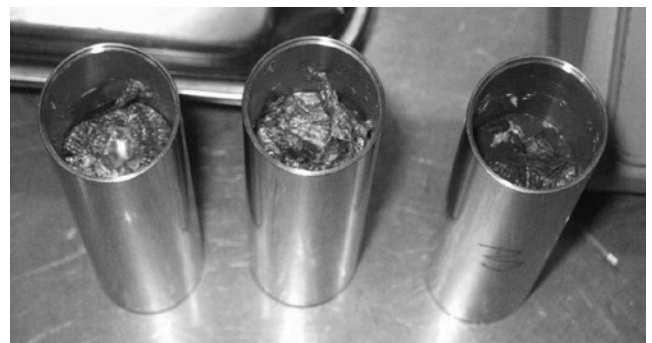
Figure 1 : Cylindrical vessels made by V-5Ti alloys with vanadium specimens fulfilled in lithium.
