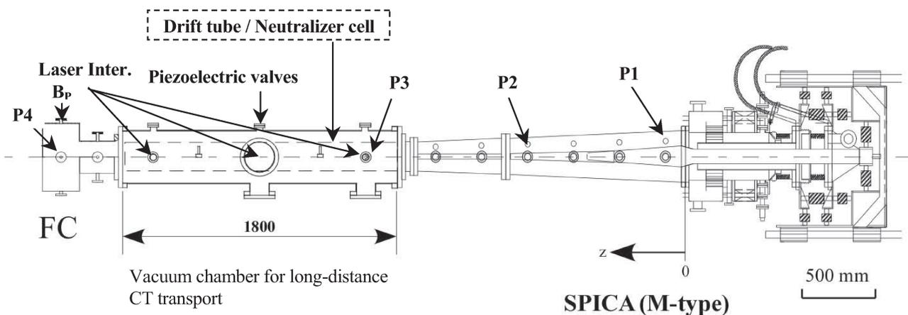
Fig. 1 Experimental setup for CT transport and production of super-high speed neutral particle flow.
