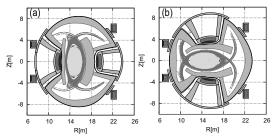
Fig. 1: Poloidal cross-sectional view of in-vessel components and supporting structure of FFHR-d1 at (a)  $\phi = 0$  and (b)  $\phi = \pi/10$ .
