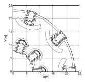
Fig. 2: Horizontal cross-sectional view of in-vessel components and supporting structure of FFHR-d1.
