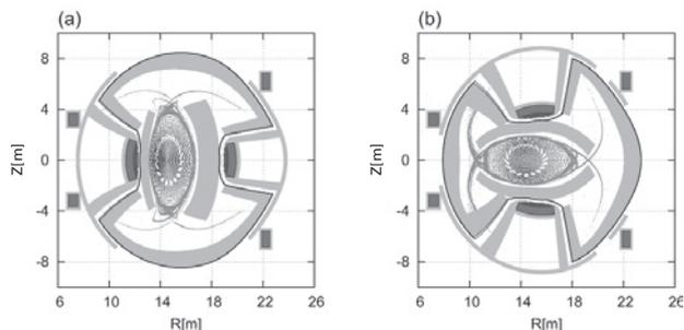
Fig. 2: Proposed basic shape of in-vessel components on (a) vertically- and (b) horizontally-elongated cross-section.
