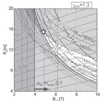
Fig. 1: Result of design window analysis for FFHR-d1. Star indicates candidate design point for FFHR-d1.
