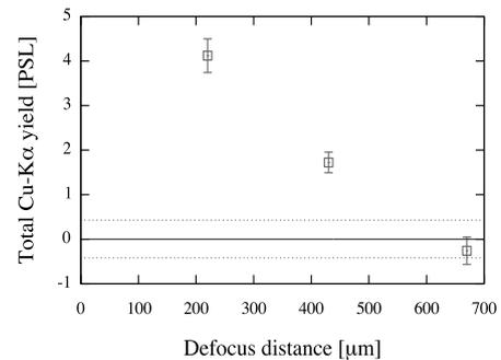
Fig. 1. Cu-K $\alpha$  intensity as a function of LFEX focusing position from the core center.
