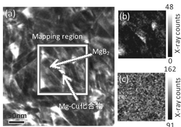
Fig. 1. STEM-EDX observation in a  $\text{MgB}_2$  wire prepared by heat treatment at 457°C for 200 h. (a) STEM high-angle annular dark-field image, (b) Cu map and (c) Mg map.
