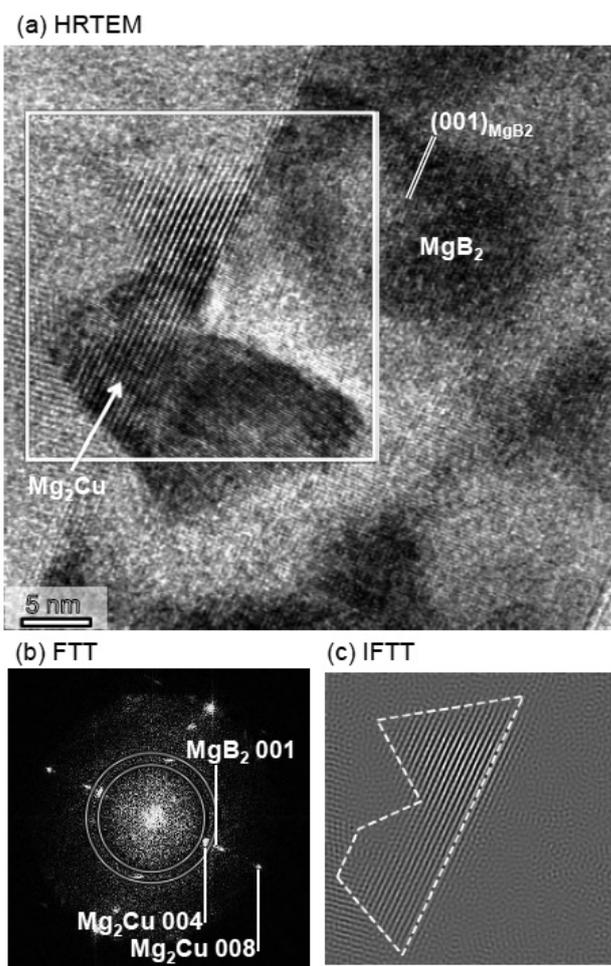
Fig. 2.  $\text{Mg}_2\text{Cu}$  phase formed on the (001) plane of  $\text{MgB}_2$  phase. (a) HRTEM image, (b) Fourier power spectrum of the square region depicted in (a), and (c) an inverse Fourier filtering image using a doughnut-shaped aperture function depicted in (b).
