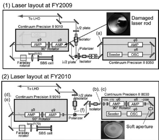
Fig. 1. Optical layout of YAG laser system
