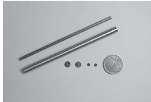
Fig. 1. Tungsten disk samples for neutron irradiation in HFIR.
