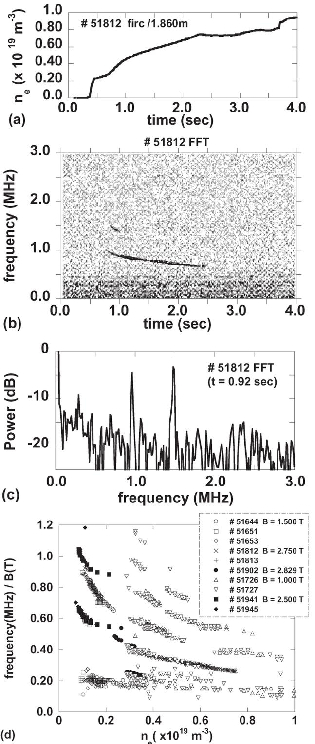
Fig. 1. (a) A plasma density as a function of time. (b) A time evolution of FFT power spectrum. (c) An example of FFT power spectrum at  $t = 0.92$  sec. (d) Frequencies of the fluctuations normalized by the field strength are plotted as a function of plasma density.
