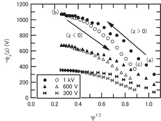
Fig. 1 Typical potential profile of CHS nonneutral plasma.
