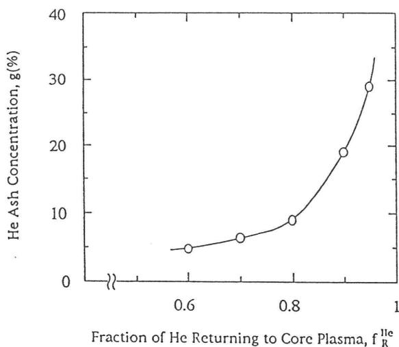
Fig.1. Ratio of helium ash concentration versus recycling ratio of helium.
