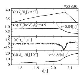
Fig. 2 Time evolution of (a)  $I_p/B_t$ , (b)  $T_e$ , (c)  $\tau_{wp}^{-1}$  and (d)  $b_{r11}/B_t$  during minor collapse.
