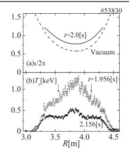
Fig. 3 Profiles of (a) rotational transform measured with MSE, and (b)  $T_{\rm e}$  before and after minor collapse. The position of arrows corresponds to  $\rho = 0.5$ .
