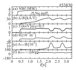
Fig. 1 Time evolution of (a) the port through power of NBI and neon puff, (b) plasma current  $I_p/B_t$ , (c) electron temperature  $T_e$ , (d) line-averaged electron density  $\bar{n}_e$ , (e) radial magnetic component of m/n = 1/1 mode  $b_{r11}/B_t$ , and (f) toroidal angle of X-point of m/n = 1/1 mode at outboard side  $\phi_{(m/n=1/1)}$ .
