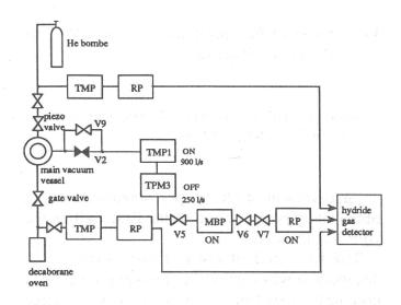
Fig. 2 JIPPT-IIU main pumping system and boronization system. During boronization the main valve V2 is closed and a small conductance valve V9 is opened.
