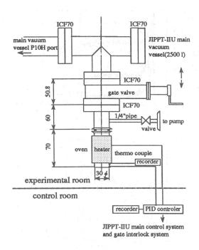
Fig.1 Vacuum system from oven to the main vessel with schematic drawings of control sytemfor boronization.
