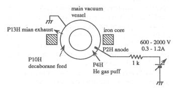
Fig. 3 Schematic diagram of glow discharge. P2H etc. means horizontal port No.2 etc..
