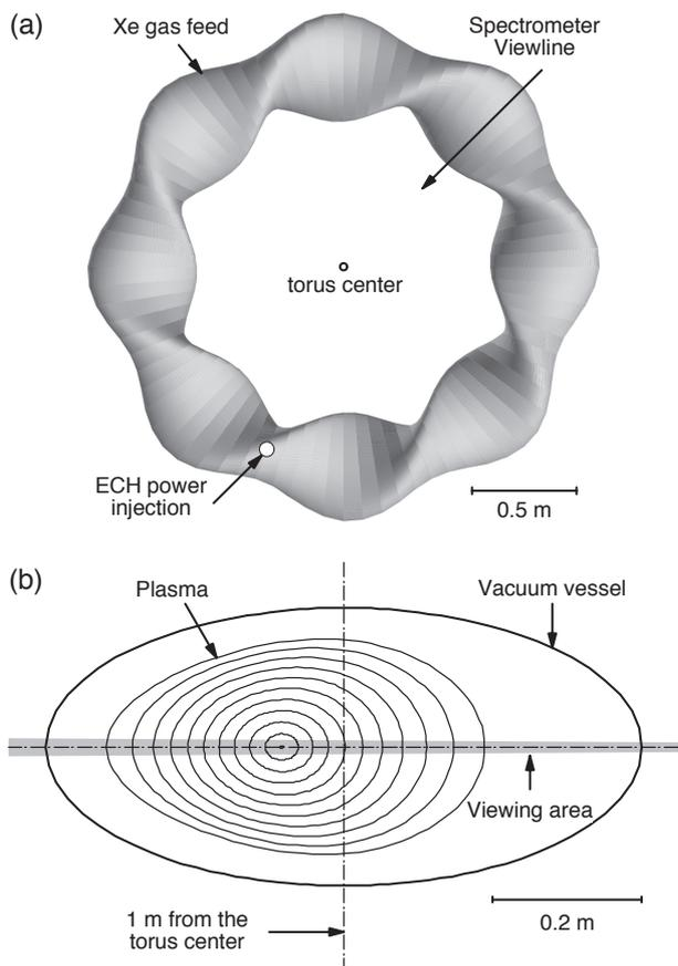
Fig. 1 (a) Top view of the standard configuration of Compact Helical System (CHS) plasma. ECH power is injected vertically from the upper viewport. (b) Cross-sectional view of the plasma and the viewline of the spectrometer.
