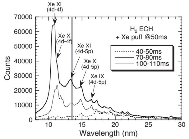
Fig. 4 EUV spectra measured before the Xe injection (40–50 ms), after the injection (70–80 ms), and in the decay phase (100–110 ms).
