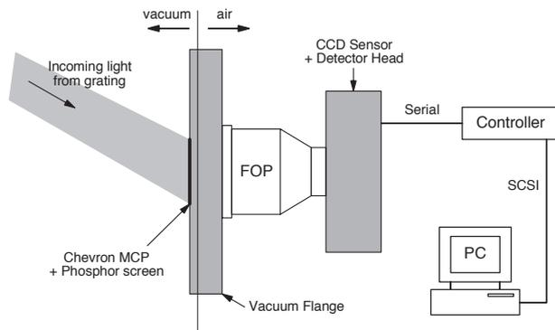
Fig. 2 Schematic diagram of the detector system of the spectrometer.
