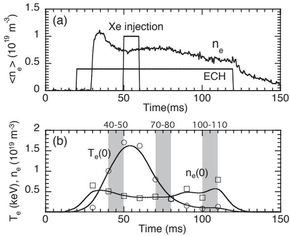
Fig. 3 Temporal variations of plasma parameters analyzed in this study. (a) Line averaged electron density measured by an interferometer, and (b) temporal variations of central electron temperature and density measured by Thomson scattering diagnostic. Gray regions are the time intervals corresponding to the spectra shown in Fig. 4.
