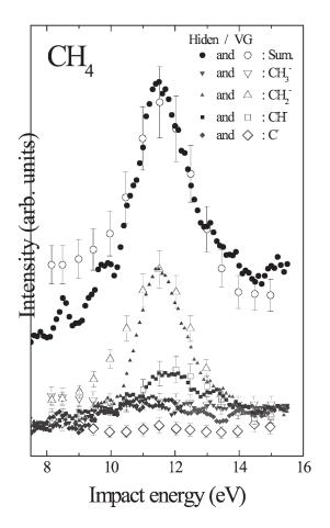
Fig. 1:  $C^-$ ,  $CH^-$ ,  $CH_2^-$  and  $CH_3^-$  formation through dissociative electron attachment to  $CH_4$ . Error bars show the statistical uncertainties in these measurements.
