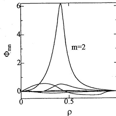
Fig.2 Fourier components of the  $n=1$  mode for smooth pressure.
