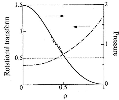
Fig.1 Profiles of rotational transform and pressure at  $\beta_0 = 2\%$ .
