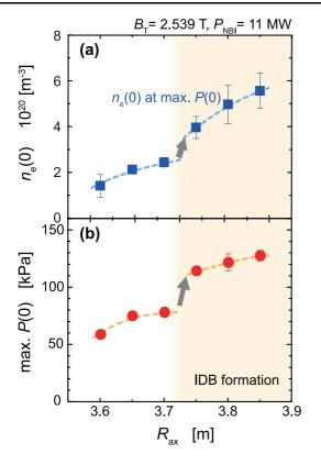
Fig. 4 Configuration dependence of (a) central electron density at the instant of maximum central pressure and (b) maximum central pressure. The magnetic field strength and NB heating power are 2.54 T and 11 MW, respectively.
