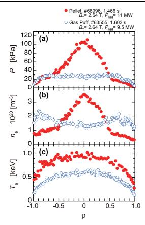
Fig. 1 Comparison of (a) plasma pressure, (b) electron density and (c) electron temperature in the gas-puff (blue open circle) and pellet (red filled circle) fueled discharges at the same magnetic configuration  $R_{ax} = 3.75$  m.
