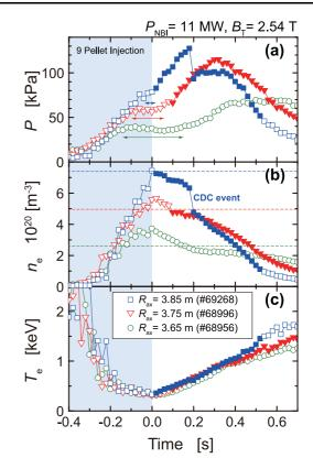
Fig. 2 The temporal evolution of (a) plasma pressure, (b) electron density and (c) electron temperature in nine-pellets fueled discharges at magnetic axes  $R_{ax} = 3.65$  m (green circle), 3.75 m (red triangle) and 3.85 m (blue square). The magnetic field strength and NB heating power are 2.54 T and 11 MW, respectively. Filled symbols denote the formation of IDB.
