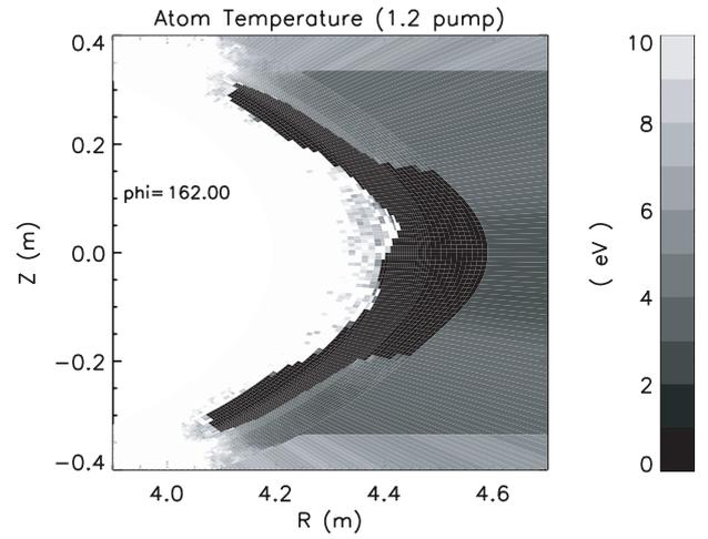
Fig. 3(a) Atom temperature profile around LID head.
