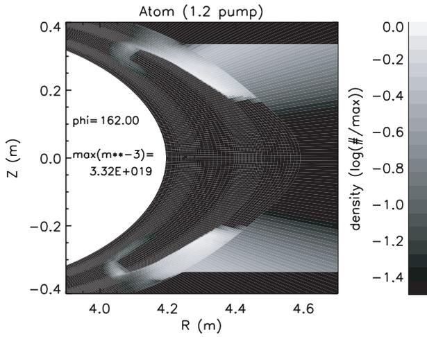
Fig. 2(a) Atom density profile around the LID head, in logarithmic scale normalized to the maximum density of  $3.3 \times 10^{19} \text{ m}^{-3}$ . The LID head is depicted with the black background.
