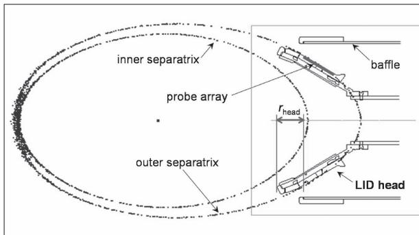
Fig. 1 Schematics of LID head and the pump duct together with the separatrix of  $(m,n) = (1,1)$  island, at  $\phi = 162^\circ$ .
