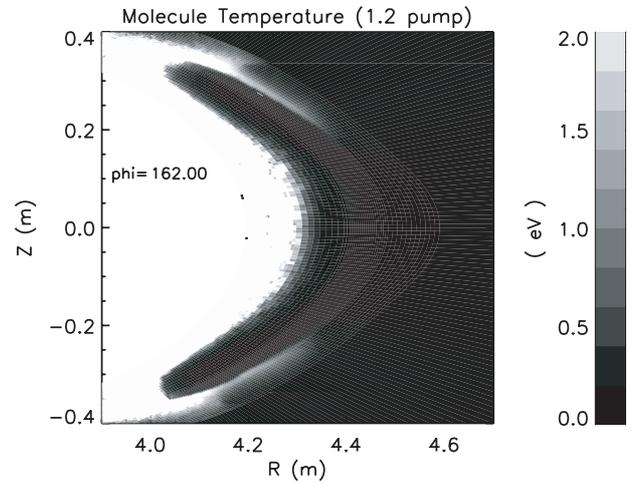
Fig. 3(b) Molecule temperature profile around LID head.
