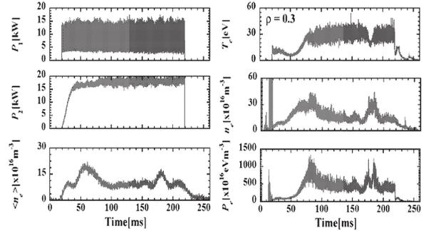
Fig. 1 Time evolutions of microwave powers ( $P_1$ ,  $P_2$ ), line averaged density ( $\langle n_e \rangle$ ),  $T_e$ ,  $n_e$  and  $P_e$  at  $\rho = 0.3$ , where the modulation frequency of  $P_1$  is 1 kHz and  $B_{t0} = 613$  G.
