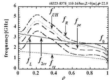
Fig. 3 Radial profiles of characteristic frequencies in the equatorial plane of the horizontally elongated section. The frequency  $f_0$  is 2.45 GHz,  $f_{pe}$  is plasma frequency,  $f_{r,L}$  are right and left hand cutoff frequency,  $f_{UH}$  is upper hybrid frequency,  $f_{ce,2ce}$  are fundamental and 2<sup>nd</sup> harmonic electron cyclotron frequency.
