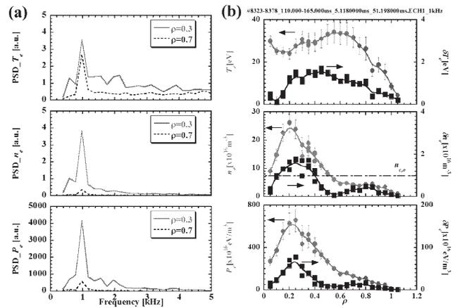
Fig. 2 (a) Power spectral densities of  $T_e$ ,  $n_e$  and  $P_e$  at  $\rho = 0.3$  and 0.7. (b) Radial profiles of  $T_e$ ,  $n_e$ ,  $P_e$  and those modulated amplitudes.
