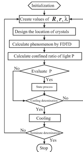
Figure 1: The algorithm for calculating optimal parameters for the design of the photonic crystal with photonic band gap.
