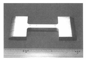
Fig. 1 Photograph of the "H" shaped YBCO bulk conductor for the prototype current feed device.
