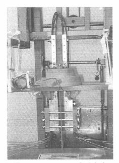
Fig. 2 The prototype current feed device assembled in the center plug of the lambda plate.
