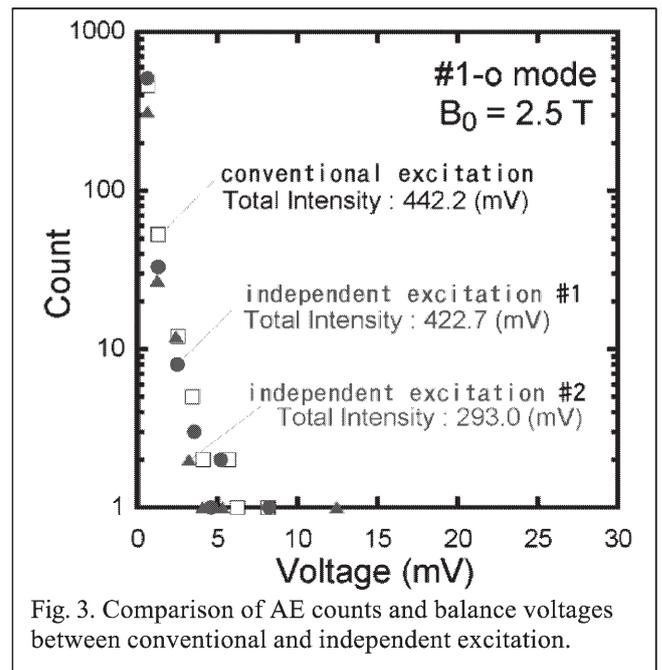
Fig. 3. Comparison of AE counts and balance voltages between conventional and independent excitation.
