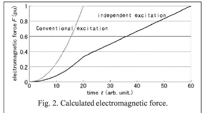
Fig. 2. Calculated electromagnetic force.
