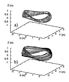
Fig. 1. Collisionless beam ion orbits in Cartesian coordinates for CHS-qa. Three-dimensional plots of orbits of (a) energetic passing H<sup>+</sup> ions ( $v_{1/}/v \sim 1$ ) and (b) toroidally trapped ions ( $v_{1/}/v \sim 0.26$ ) with an energy of 38keV in  $B_t$  of 1.5T.
