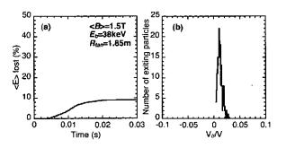
Fig. 2. (a) Time evolution of  $\langle E \rangle$  lost (%), (b) Number of exiting beam ions as a function of pitch angle  $v_{ll}/v$
