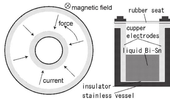
Fig. 2. Test section of experimental set-up.
