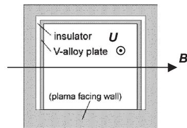
Fig. 1. three-surface and multi-layer coated channel.
