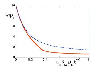
FIG. 1. The width of the magnetic island as a function of the plasma beta value. The parameter  $\delta$  is fixed,  $\delta/\rho_b=10$ . The dashed line indicates the suppression by the bootstrap current effect and the solid line includes the ion polarization drift. We simply choose  $2|\Delta'_0|=1$ ,  $L_q/L_p=3$ , and  $a_{pc}=a_{bs}$ .
