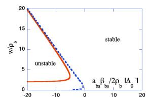
FIG. 4. Magnetic island width as a function of the plasma pressure gradient when the bootstrap current is in the counterdirection. We take  $\delta$ =0 in this case. The solid line shows that the ion-polarization current has a stabilizing effect,  $a_{\rm pc}$ =| $a_{\rm bs}$ |. The dashed line indicates the case that it is destabilizing for  $a_{\rm bs}$ <0 ( $a_{\rm pc}$ = $a_{\rm bs}$ ). (Other parameters are the same as in Fig. 1.)
