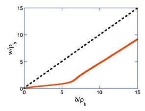
FIG. 2. The width of the island as a function of the intrinsic island width  $\delta$  for a fixed value of the plasma pressure,  $a_{\rm bs}\beta_{\rm bs}$ =0.3 and  $r_s/\rho_b$ =50. (Other parameters are the same as in Fig. 1.)
