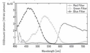
**Fig. 2.** Count of the color CCD detector (16 bits) per photon measured using the liquid-crystal-based tunable Lyot filter spectra camera system (Fig. 1). The red and green peaks below 450 nm are attributed to the leak-bands of the Lyot filter, so the CCD count of the red layer below 450 nm cannot be used as a calibration function.
