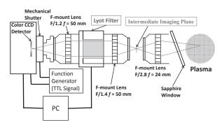
**Fig. 1.** Schematic of liquid-crystal-based tunable Lyot filter spectra camera system.
