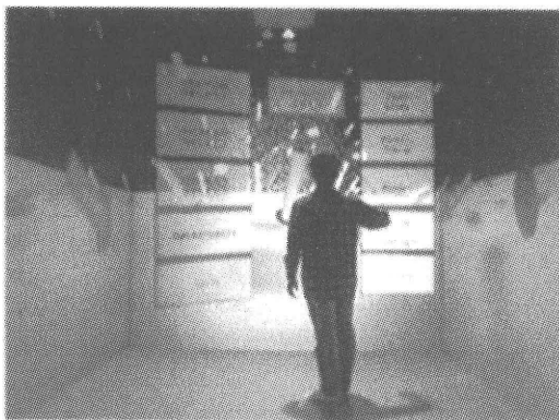
Fig.1 Menu system of VFIVE. The viewer shoots menu panels to choose visualization modules.
