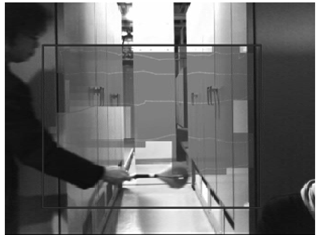
Fig. 1. Compliance distribution of protection guideline in the vicinity of entrance of passage (ICNIRP 1998).
