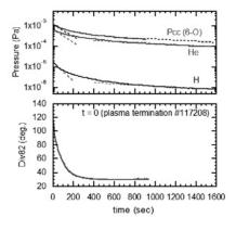
Fig. 2. Time evolution for pressures and divertor temperature in the vacuum vessel just after high-performance long-pulse discharge.
