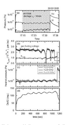
Fig. 1. Hydrogen and helium pressure, gas fueling, line averaged electron density, neutral pressure ( $P_{cc}$ ) and divertor temperature during the long-pulse discharge.
