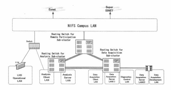
Fig. 1 Block diagram of new LHD-LAN
