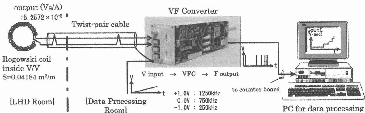
Fig.1 Schematic configuration of plasma current measurement in LHD
