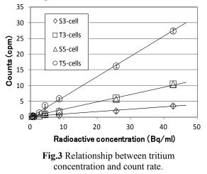
and a S3-cell, where both lines for T3-cells and a S5-cell are almost overlapped. Since the steep angle corresponds to radiation sensitivity, T5-cells are most sensitive. The results suggest that relation between count rates and concentrations was definitely linear above a few Bq/ml. Taking accounts these results the tritium water monitoring system could be improved in the future study.
