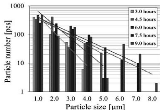
Fig. 3 Distributions of size on carbon dusts with discharge durations of 3.0, 4.5, 6.0, 7.5 and 9.0 hours.
