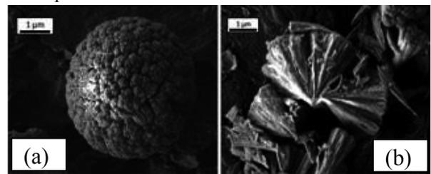
Fig. 2 Surface (a) and inner (b) structures of carbon dusts after hydrogen plasma discharge.
