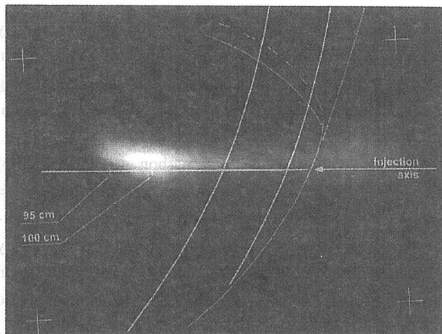
Fig. 1. CCD image of the pellet cloud in Li II light overlapped with geometry contours. Two values of major radius are shown ( $R_{ax}=92.1$  cm).
