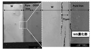
Fig. 1: Cracks formed in the W-ODSS joint produced with a double layered insert Fe/amorphous after bending test..
