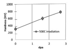
Fig. 2: Dose dependence of irradiation hardening of VPS-W irradiated at 773K.
