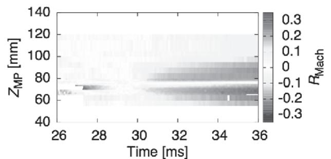
Fig. 2 Time evolution of the radial profile of the poloidal flow measured by the multi-points Mach probe
