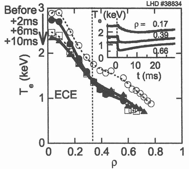
Fig. 1: Time evolution of electron temperature profile measured with heterodyne radiometer. The TESPEL is injected at  $t = 0\text{ms}$ .
