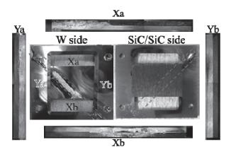
Figure 2. Surface Morphology after Plasma Exposure
