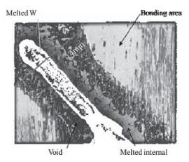
Figure 3. The Result of Ultrasonic Test
