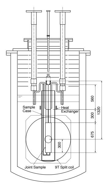
Fig. 1. Set up of an ITER-TF joint sample in the conductor test facility with 9 T split coils.
